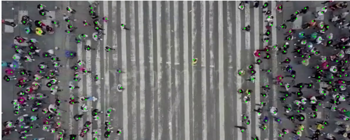
Fig. 2. Trajectories were extracted from real data video by tracking pedestrian's heads with an open computer vision software library. At a second stage, trajectories were cleaned from periodic walking movements using a Kalman filter and then re-sampled at 72 frames per second.
