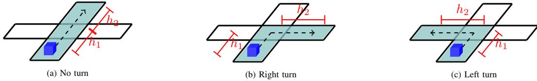
Fig. 3: Schematic representation of the desired trajectories (dashed line) the agent (blue cube) should follow: (a) no turn required, (b) right turn, and, (c) left turn. The teal tiles represent the lane components the agent will trace. The agent is required to move a distance  $\sim h_1$  up to the intersection and a distance  $\sim h_2$  thereafter to reach the target.
