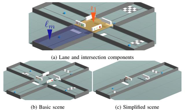
Fig. 1: Stills from the game scene: (a) shows a lane component  $\ell_m$  shaded in blue and intersection component  $\iota_1$  shaded in orange, (b) shows the basic crossroad scene and (c) the simplified scene.
