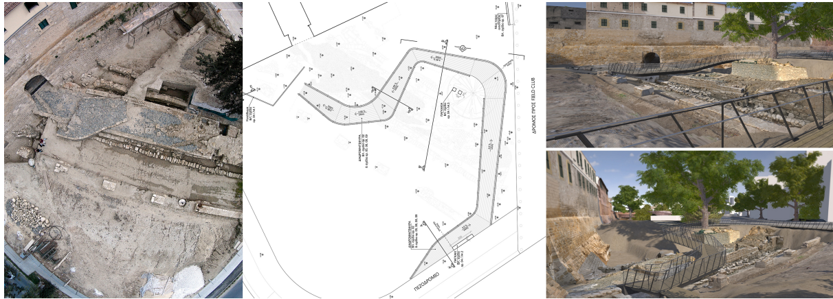
Figure 2: (left) Aerial view of the site from the drone mapping process; (middle) proposed site plan; (right) visualization of the proposed walking platforms as seen in the virtual environment.
